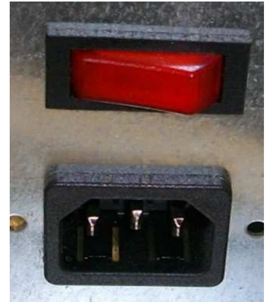
Fig 5.6a: Power supply connection point
