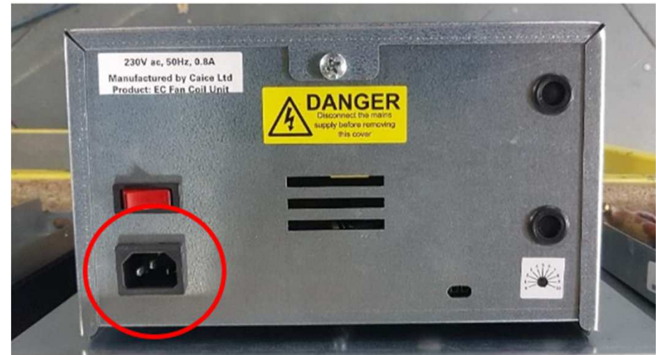
Fig 5.6c: Power supply connection point
