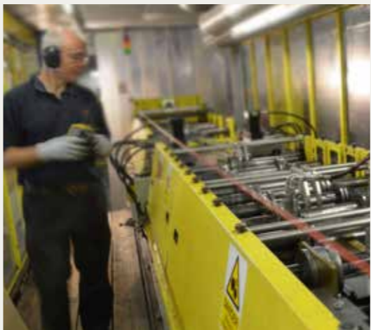
Splitter Line A bespoke piece of machinery at our product centre for automated manufacture of splitters.
